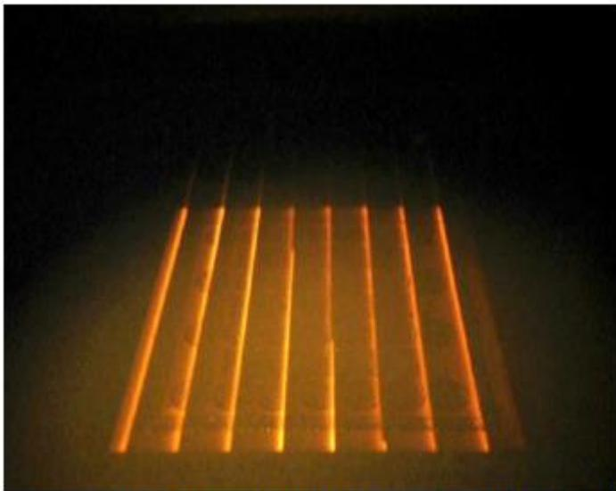
**Figure 5** EBM Multi-beam Technology- Melt pools for a layer
