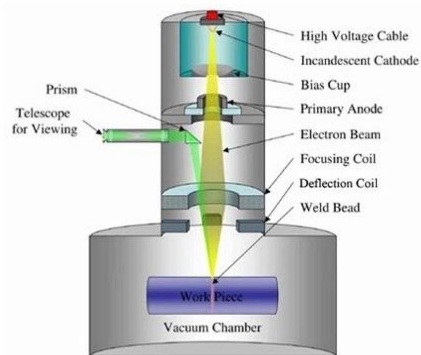
**Figure 2** A schematic overview of the EBM technology (<http://3dprintingfromscratch.com/common/types-of-3d-printers-or-3d-printing-technologies-overview/#ebm>).
