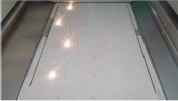
**Figure 3** Real time picture of 4 lasers, 4 scanners SLM system (11)
