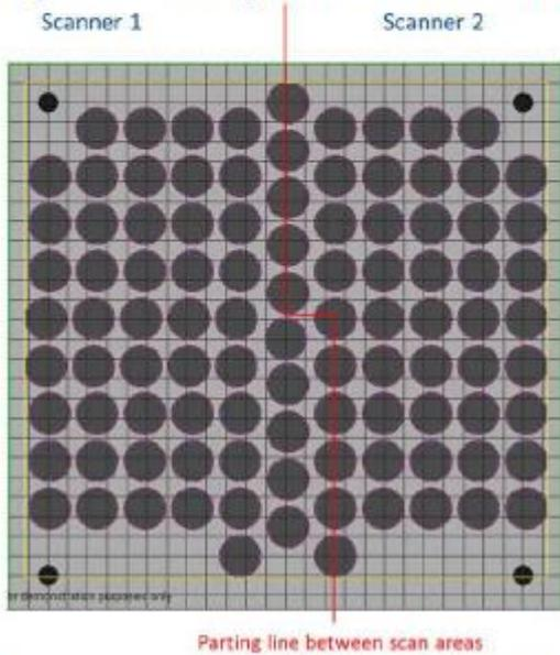
**Figure 4** Schematics of designed overlap between 2 lasers – 2 scanning system (11)
