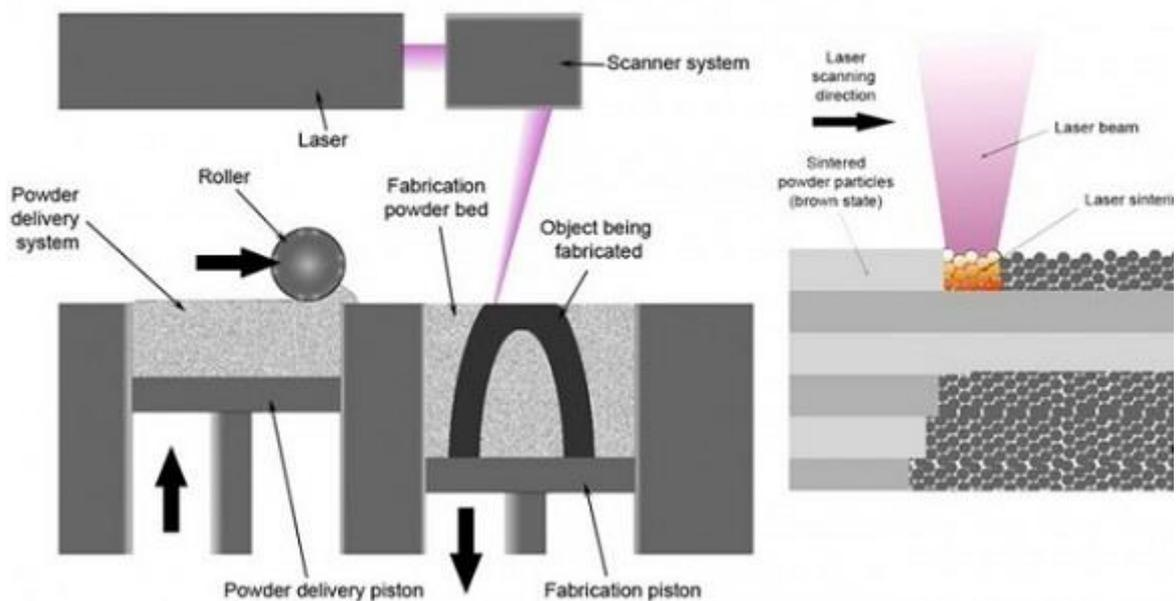
**Figure 1** Schematic overview of the SLM technology
