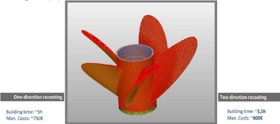
**Figure 6** Marine propelling screw AlSi12 / 350 Watts 50 micron layer thickness. Build time 3.5 hours. X/Y: 100mm, Z: 70mm (Ritt, 2012)
