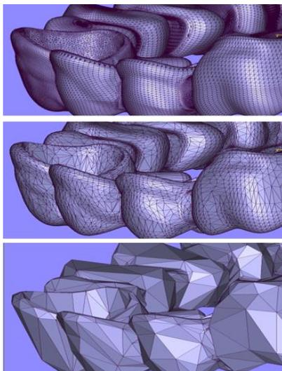
**Figure 3** Three levels of accuracy of the STL file
