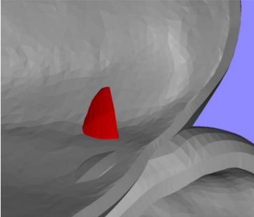
**Figure 4** Detail of a normal vector of an STL file
