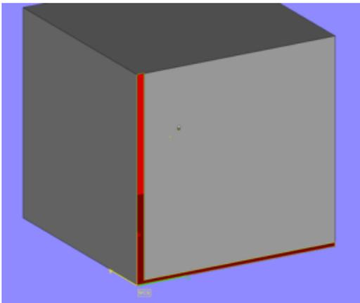
**Figure 5** Detail of a non-manifold STL
